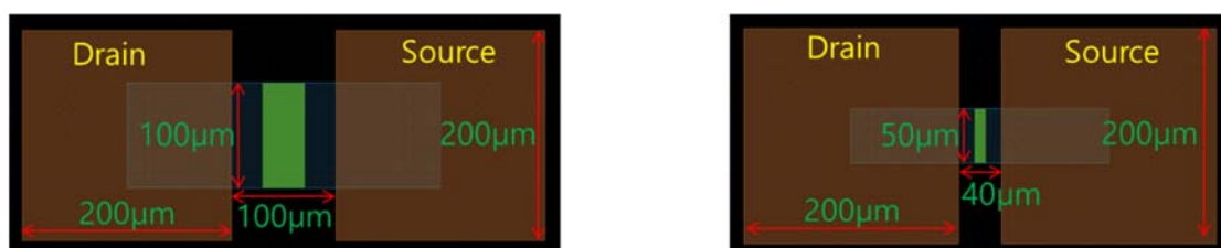
Figure 3.2 Mask design for the plasmon FETs with two different W/L of gold NPs. 100µm by 100µm (left) and 50µm by 40µm(right).
