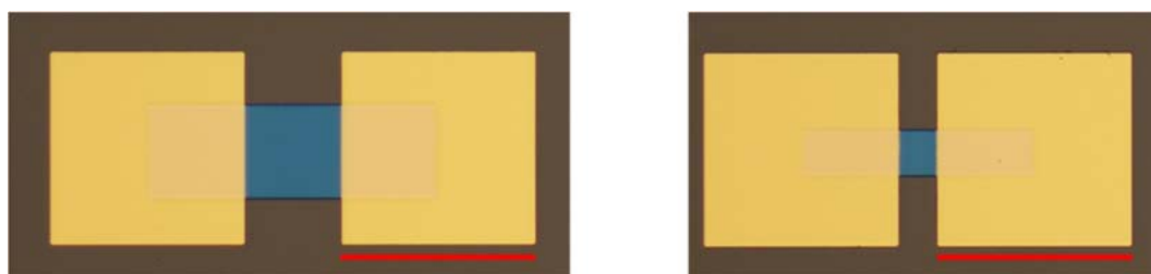
Figure 3.6 Microscopic pictures of fabricated thin film transistors with W/L 1/1 (left) and W/L 5/4 (right) on a silicon substrate. Scale bar is 200 \mu m.
